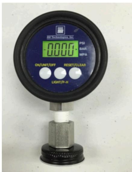
**Fig. (4).** Pressure gauge integrated with container cap to measure headspace pressure of a bottle.
