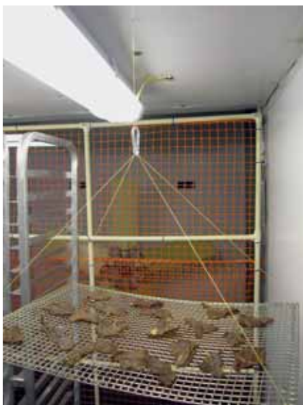
Fig. (1). Weigh pan setup in dehydrator for continuously monitoring weight loss of product.
