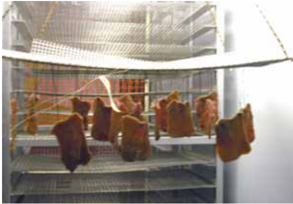
Fig. (2). Vertically oriented product suspended from the weigh pan using wire hooks.
